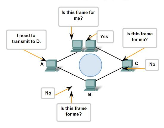
Purpose of encapsulation of data into frames: to facilitate the entry and exit of data on the media!
