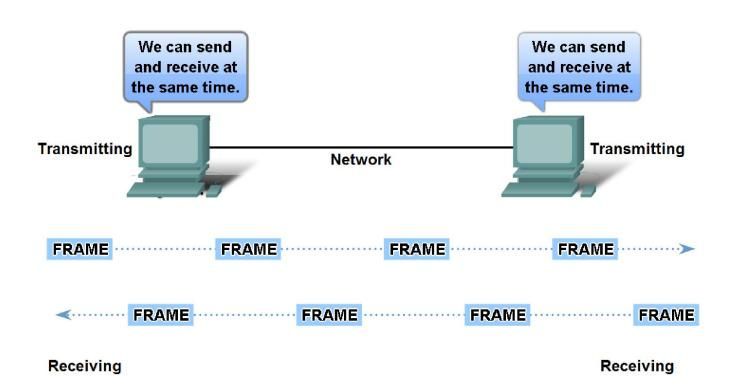
Logical topology – way a network transfers frames from one node to the next. This is what the data link layer 'sees' when controlling media access. These are virtual connections
